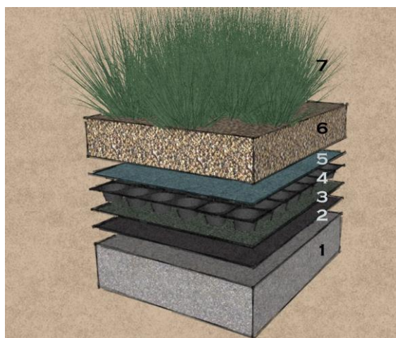
Figure 1 – Green Roof Stratification
