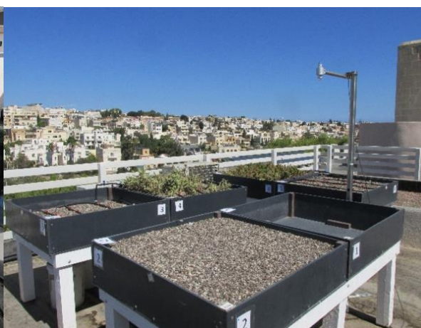
Figure 66 1m x 1m test trays made from recycled plastic
