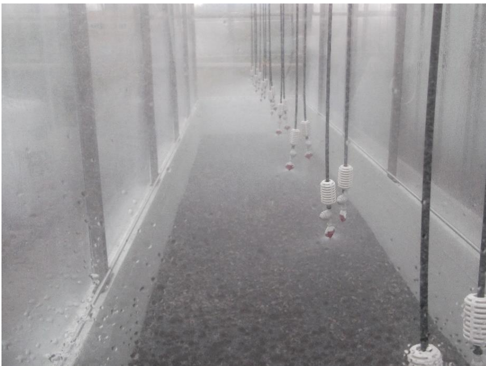
Figure 55 High intensity rain test in progress within the rain chamber
