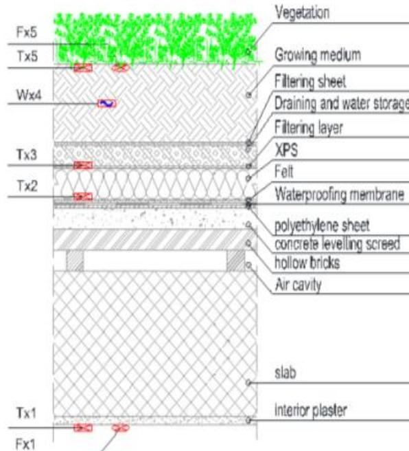
Figure 42 Green roof layers in Politecnico: the monitored plot has the same drainage and filter layer, the same growing media as well as its depth (10 cm) and vegetation as the green roof in Minopri
