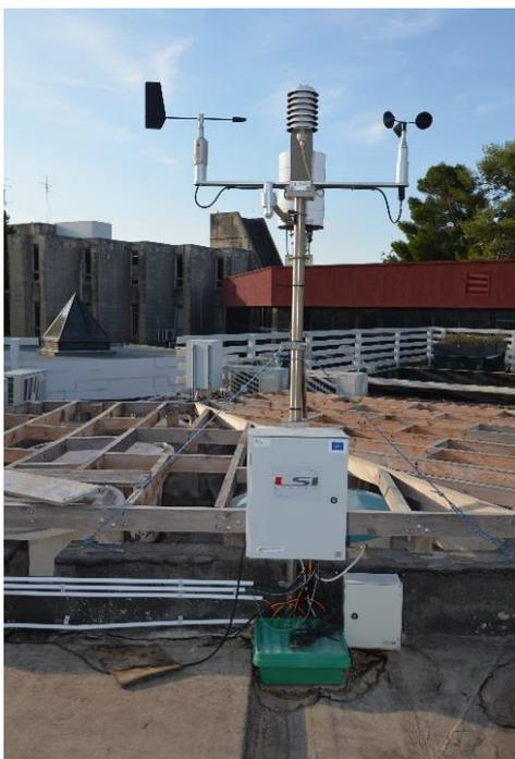
Data from each of the sensors was recorded at intervals of 10 minutes. In order to provide an early indication of the thermal insulation potential of the green roof a thermal imaging camera was used to sample the area around the two sets of sensors before the polystyrene box was fitted. (Figure 29)
