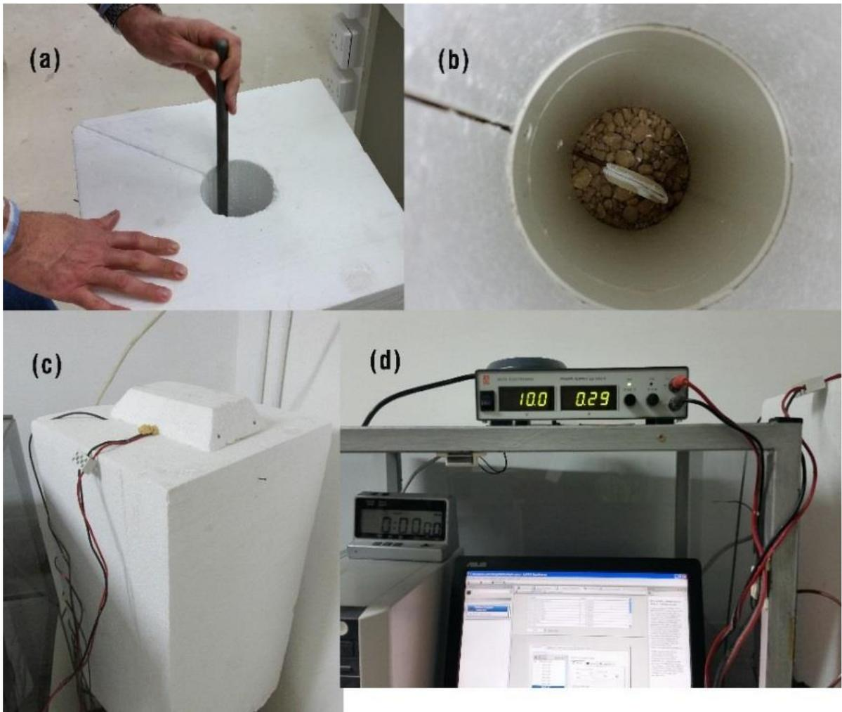
Figure 52 Experimental set-up to assess the thermal resistance of the various elements of the core taken through the roof slab above the Faculty of the Built Environment.
