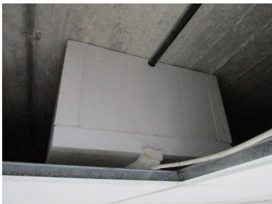
Figure 25 Photograph of Polystyrene box placed over the sensors attached to the ceiling
