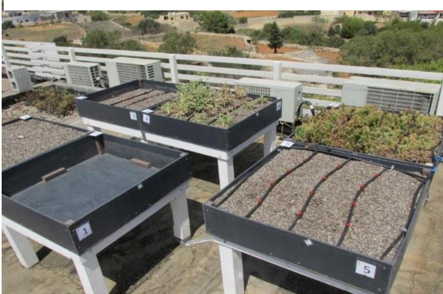
Six Test trays were constructed from 12mm recycled plastic boards to form 1000mm x 1000mm x 250mm containers. These were supported on timber benches so as to provide access in order to attach the thermocouples to the sub-surfaces of the trays. Figure 4.5 below shows the general arrangement of the test trays. A 50mm thick sheet of expanded polystyrene was placed beneath the timber benches to cover the thermocouples to prevent the influence of fluctuating ambient air temperatures.
