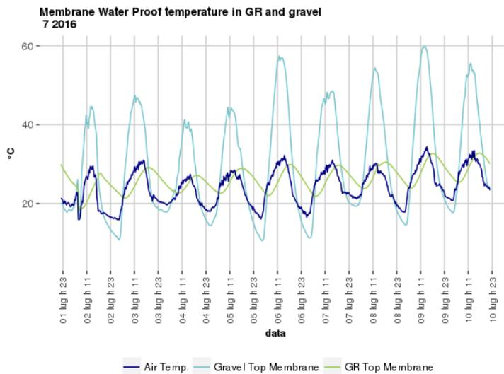
Figure 44 Summer membrane temperatures: extract of a ten day period in July 2016
